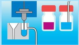
The syringe is filled with rinsing solvent, the plunger moved past the side connection and some additional rinsing solvent is aspirated off.
