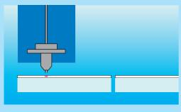
Prior to the first application from a newly filled syringe, a small sample volume is pre-dosed onto a waste plate in order to generate reproducible conditions at the needle tip. Pre-dosage is effected in the same way as intended for sample application, i.e. by contact spotting or by spray-on technique.
