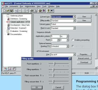
The ATS4 is controlled by the winCATS Planar Chromatography Manager, an easy to use Windows application designed to monitor all steps in the TLC process, from sample application via chromatogram development, etc. to evaluation and result documentation in conformity to GMP/GLP. Like other computer controlled CAMAG instruments the ATS4 communicates with winCATS via a software interface called "EquiLink"
