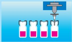
The septum punch is retracted before the needle to ensure that the outside of the needle is wiped off by the tightly closing septum.
