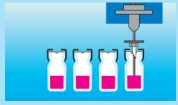
An application sequence starts with the take-up of the sample. The septum is punched and the needle lowered into the sample vial through the septum punch. Then the syringe is filled with sample solution.
