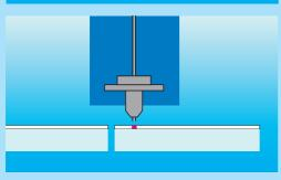
The syringe moves to the programmed position of the plate and starts application of the desired sample volume. If several applications of the same sample have been programmed, these are applied in sequence from the same syringe filling, provided the remaining volume is sufficient. Otherwise the syringe is automatically refilled.
